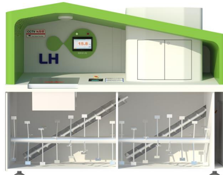
Food wastes disposal system
